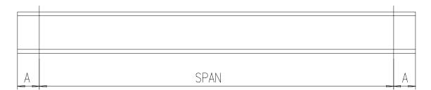
The bridge beam length for UC or UT16 end truck may be estimated by using the formula of SPAN + 2A. SPAN is horizontal distance center-to-center of runway rails and dimension "A" is the length from crane wheel center to the outside edge of the beam connection plate or bridge beam.
